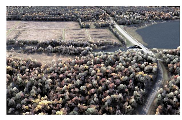
Lidar Point Cloud Colorized by Photo
