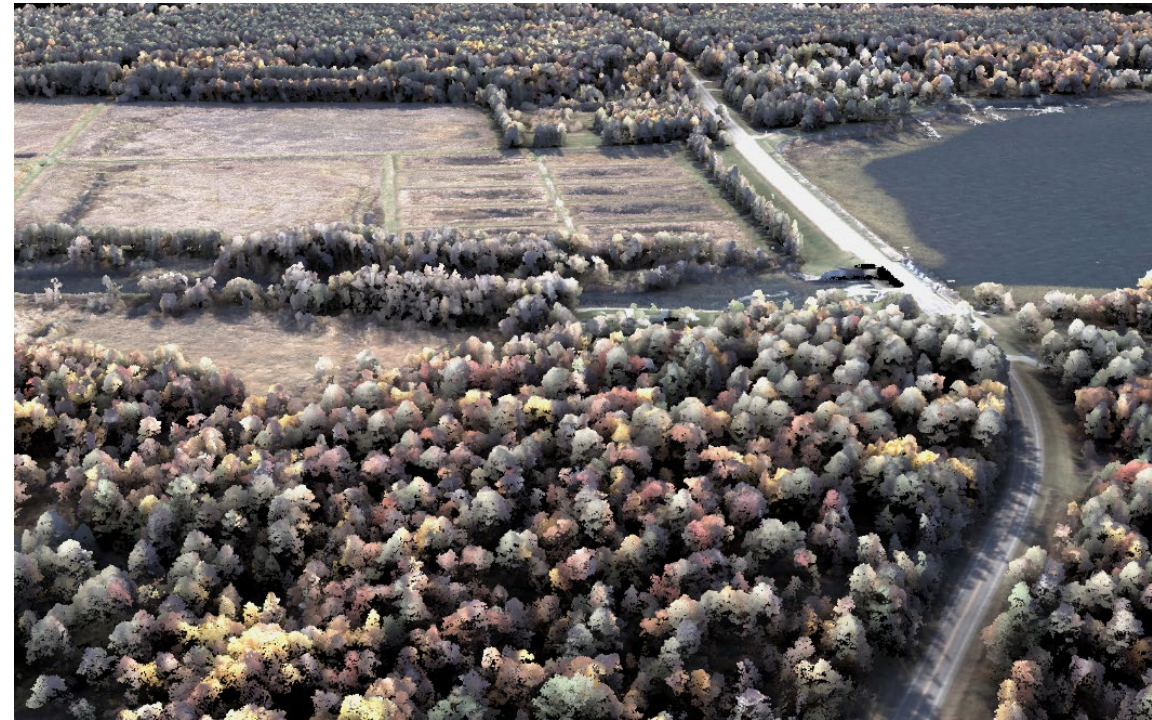
Lidar point cloud colorized by photograph pixel colors
