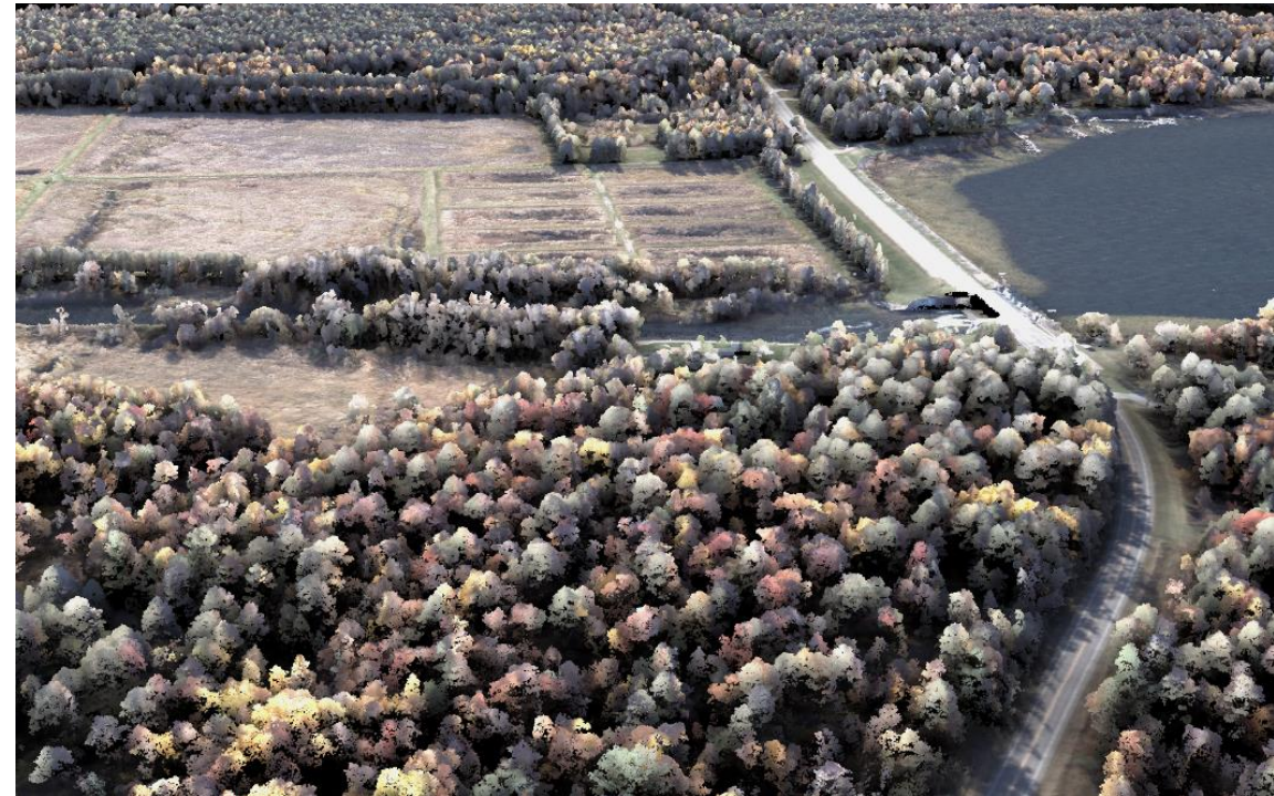
Lidar point cloud colored by photograph pixel colors
